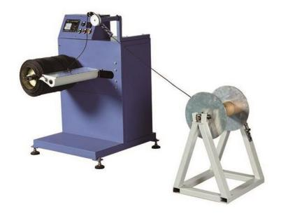
该机器主要配套纸绳机使用,以纸绳机的绳卷为原料,通过机器轴心的高速旋转,将绳卷在一端快速释放并在另一端复卷一遍,既能扩大最终绳卷的外径和绳卷中心的内径,又能消除原有绳卷中可能存在打结现象,从而确保纸绳在后续生产中大大提高生产效率和质量 This machine mainly support twisted paper rope machine. This machine takes the paper rope roll produced from twisted paper rope machine as the raw material, releases the roll on one shaft and twines it on the other shaft on the machine. This machine
